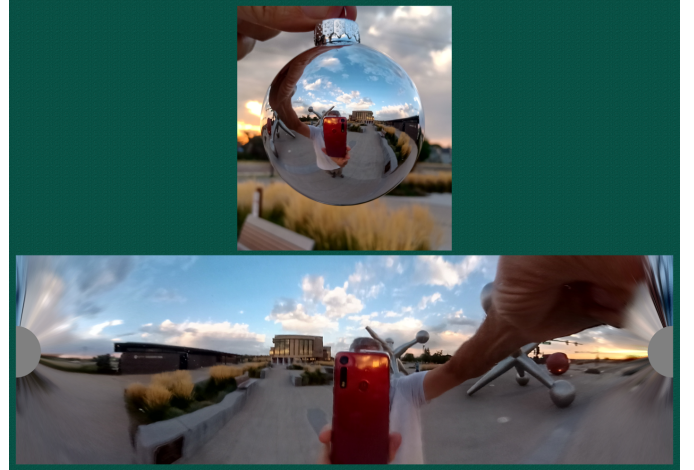
Figure 1. Simple reflective optical system comprising perspective camera viewing a reflective spherical ball. The top portion is an image directly recorded by a smartphone camera while pointed toward a front-silvered spherical ornament. The bottom section shows a restored image created with the formulae presented herein. The rendered image is produced by projecting restored ray directions onto a virtual cylindrical screen.
