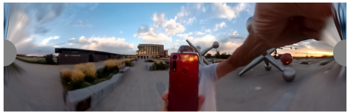
Figure 6. Cylindrically rectified image generated from the source image shown in figure 5. The geometry of this image is generated using a vertical cylinder centered on the sphere. Rows of image pixels correspond to constant elevation value along this cylinder, while columns of images correspond to constant azimuth direction.
